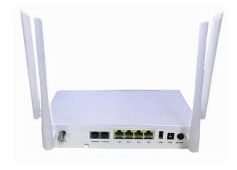
ITU-T G.984.x GPON IEEE802.3ah GEPON Standard 1.25G upstream 2.5G/1.25 downstream RTL9607 600Mhz CPU Multi-WAN Route/Bridge
